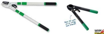
To operate, open the blade fully to grab the material to be cut which also resets the ratchet mechanism. Close the blade till it will not cut any further. To fully utilize the mechanical advantage of the ratchet, the handles should then be **opened slowly** till the mechanism activates **one click** only then shut again to apply the greatest cutting force on the material being cut. This action may need to be repeated a number of times till the cut is complete.
