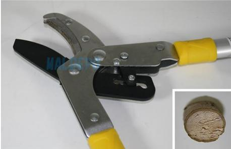
When selecting loppers we have found that the **anvil style blade** with a **ratchet** system tends to provide the most effective cutting results. The cut should be made square across the stem or root. The anvil blade will reduce the likelihood of the blade twisting and potentially snapping.
